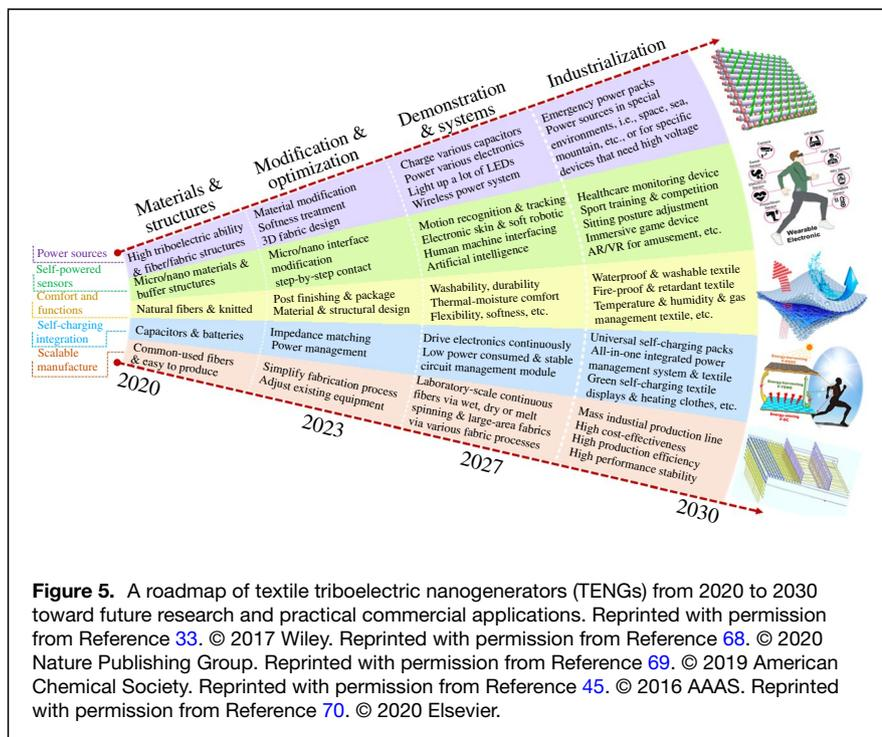
**Figure 5.** A roadmap of textile triboelectric nanogenerators (TENGs) from 2020 to 2030 toward future research and practical commercial applications. Reprinted with permission from Reference 33. © 2017 Wiley. Reprinted with permission from Reference 68. © 2020 Nature Publishing Group. Reprinted with permission from Reference 69. © 2019 American Chemical Society. Reprinted with permission from Reference 45. © 2016 AAAS. Reprinted with permission from Reference 70. © 2020 Elsevier.
